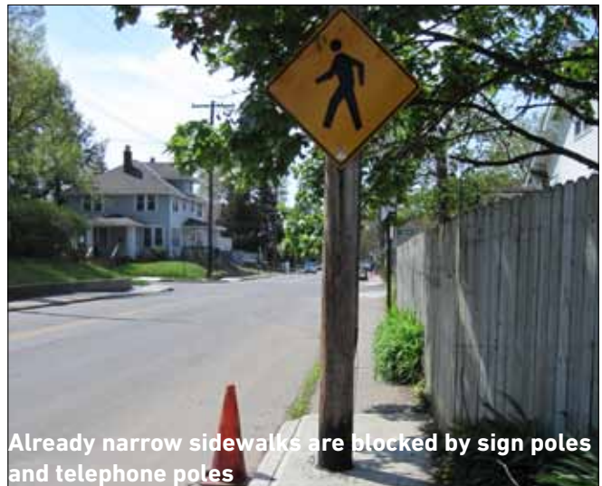
The lack of a defined parking lane or a centerline creates a visually wider street that encourages speeding
